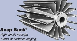
encased in a steel jacket, displaces upon belt contact. When belt contact is broken, the rubber actually "snaps back" to its original height automatically cleaning itself.
